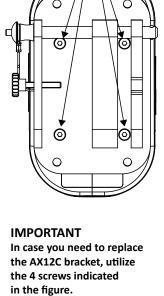
In case you decide to remove the AX12C bracket (because it is not needed), put back the screws in the threaded holes as shown in the figure, in order to avoid air leakage.
