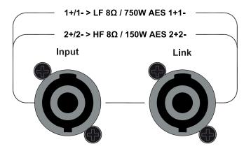
**LINK** - Power output in parallel with the INPUT socket for connecting the unit to another speaker. The number of AX2010P cabinets that can be connected in parallel depends on the amplifier load capacity.
