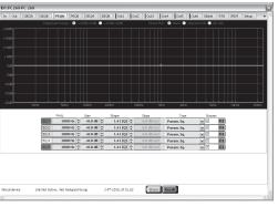
**PEQ:** this is a full parametric 5-band equalizer on the processor's inputs. Each filters can be set also as shelving, notch, allpass, high-pass and lo-pass, so this equalizer can be used to optimize the system response according to the environment characteristics, including temperature, humidity and absorption due to the audience.
