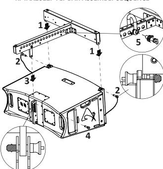
When lifting the system always proceed gradually step by step, paying attention to secure the fly bar to the box (and the box to the other boxes) before pulling up the system: this makes easier to insert properly the locking pins. Also when the system is released down, unlock gradually the pins.
