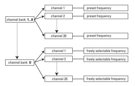
Each of the channels in the channel banks "1" to "8" has been factory-preset to a receiving frequency (see enclosed frequency table). These receiving frequencies cannot be changed but have been preset so that e.g. countryspecific regulations on frequency usage are taken into account. The channel bank "U" (user bank) allows you to store your selection out of 1,440 receiving frequencies that are freely selectable within the preset frequency range.
